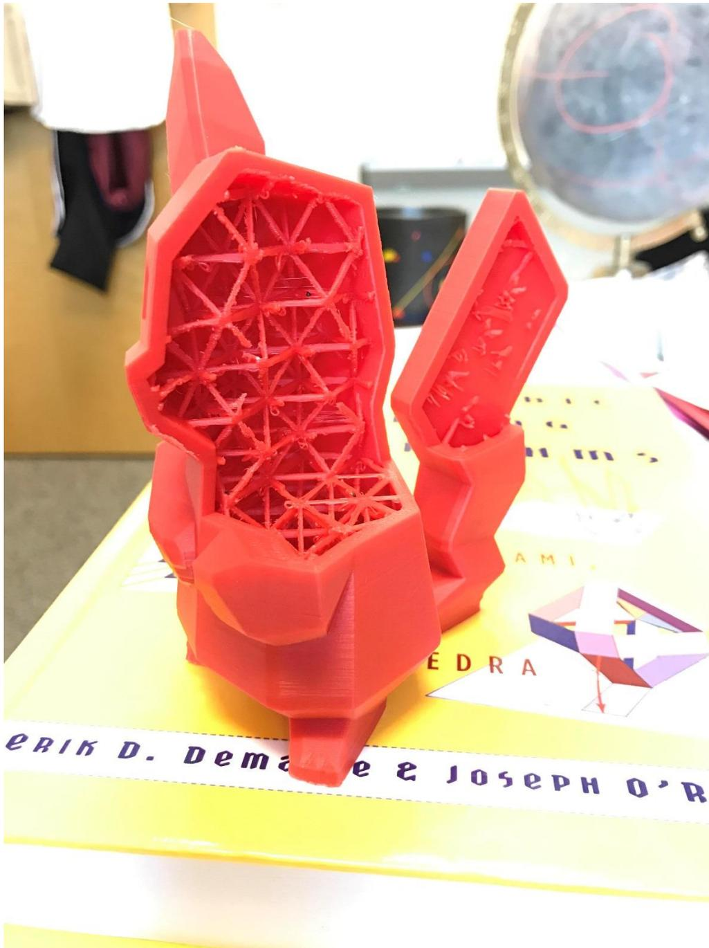
Figure 4: 3D Print using infill structure generated by sphere packing.
